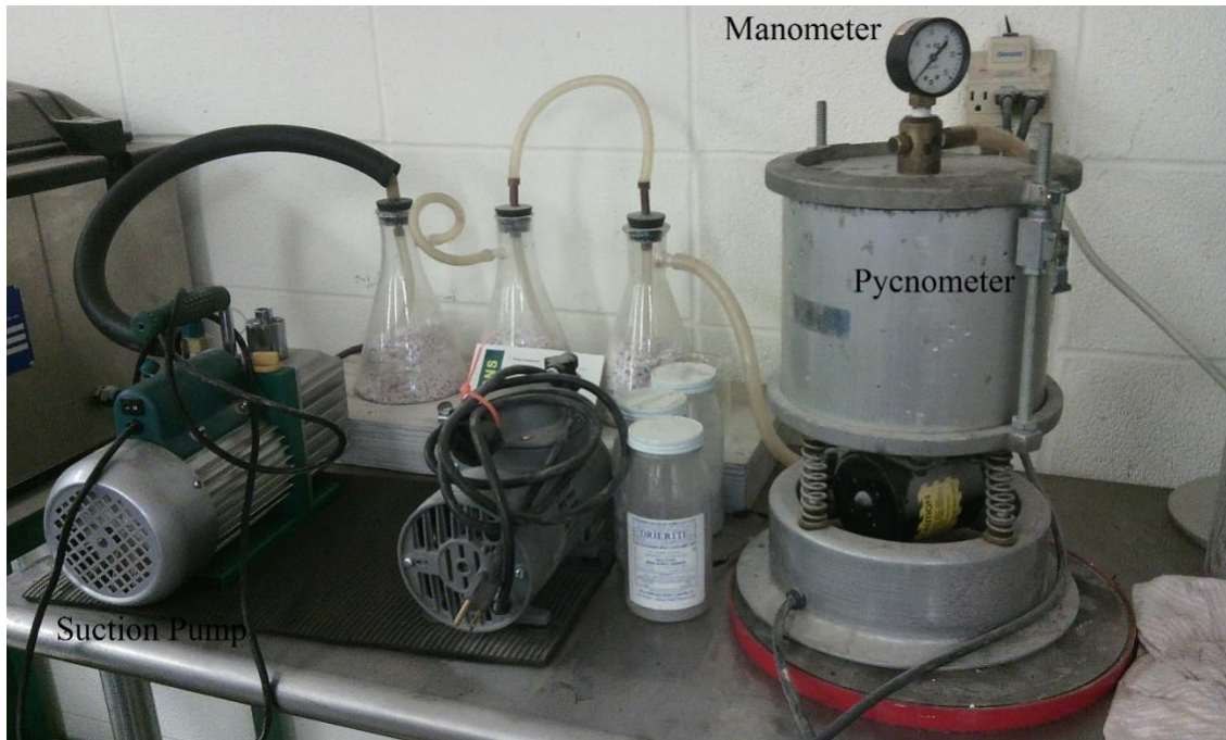
Figure 4: Apparatus for measuring ‘Rice Specific Gravity’
