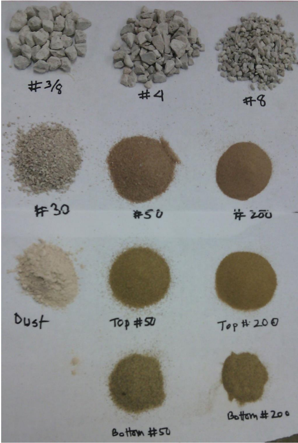
Figure 2: Different sizes of aggregates used in this study (Buda aggregates with Top and Bottom mine tailings)
