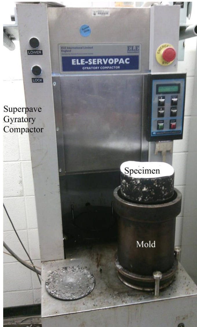
Figure 3: Superpave Gyrotory Compactor with freshly compacted test specimen
